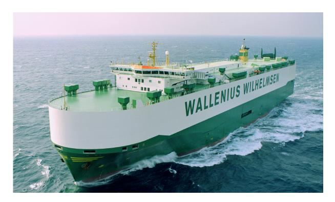
The PCTC (Pure Car Truck Carrier) m/v DON PAS-QUALE has a capacity of 7,194 cars or a combination of 3,700 cars and 600 trucks. DON PASQUALE is a sister ship to DON QUIJOTE and DON CARLOS. The ship is built to the highest class of Lloyd's Register
